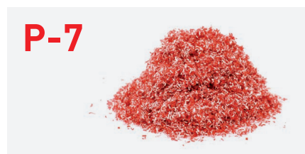
P-7 Recommended for data carriers with strictly confidential data in case the highest security precautions have to be respected. (For example particles 0.8 x 5 mm).
