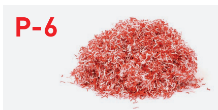
P-6 Recommended for data carriers with secret data in case extraordinarily high security precautions have to be respected. (For example particles 0.8 x 12 mm).
