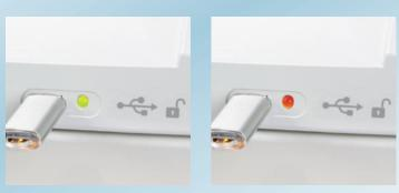
It is possible to secure the paper stack inserted into the magazine against unauthorized access by using the **Lock-and-Go function**. To this end, an individual security code is saved on a USB medium per stack processing. After starting, the shredding process can only be interrupted by the owner of the USB medium.
