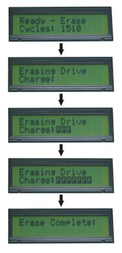
**Note:** After degaussing, hard drives should not be not be reused as they are stressed in the erasure process. Some backup tapes may not be reusable after degaussing due to the servo track being erased.
