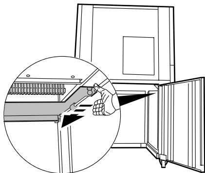
Push back the conveyor belt into the machine.
