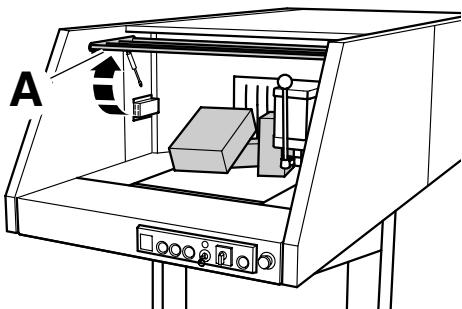
The grid (A) can be lifted to remove jammed paper.
