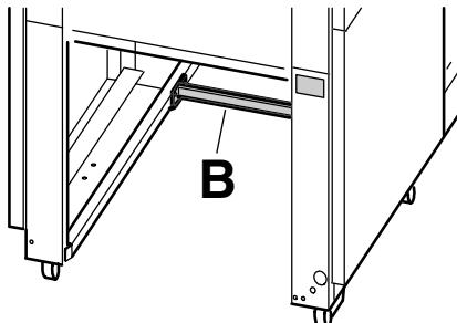
Remove the back transport safety device (B).
