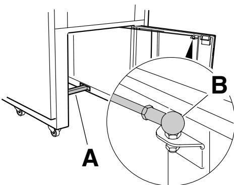
If the machine is to be operated with a waste cart the rear transport safety device (A) and tie-bar (B) must be re-assembled. To assemble follow the same instructions in the reverse order.
