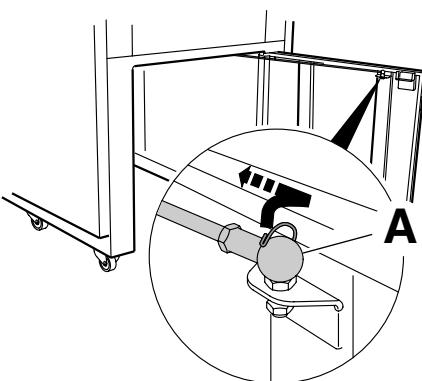
Remove the springs from the ball-ends (A) on both sides.
