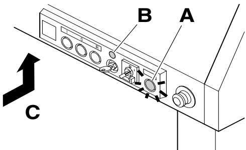
Yellow pilot light (**A**) illuminates, green light (**B**) is out → Conveyor belt is overloaded. Press the motor protection switch (**C**) after approx. 5 minutes.
