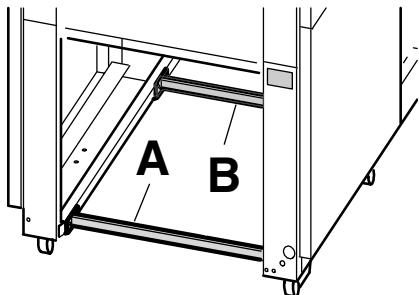
The transport safety device (**A**) and (**B**) must be mounted when the machine is transported lengthwise. The machine must be transported from the rear.
