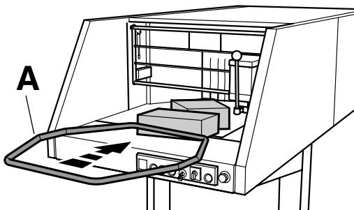
Material not caught by the shredding mechanism must be pushed with the pusher (A).
