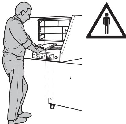
This machine is constructed for "one man operation" only!
