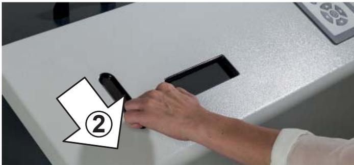
Pulling the slide (2) will allow the material to be discharged into the cutting unit.
